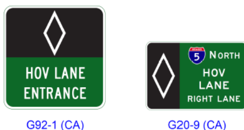
Figure 2G-6 (CA). Guide Signs for Direct Entrances to Preferential Lanes From Another Highway
