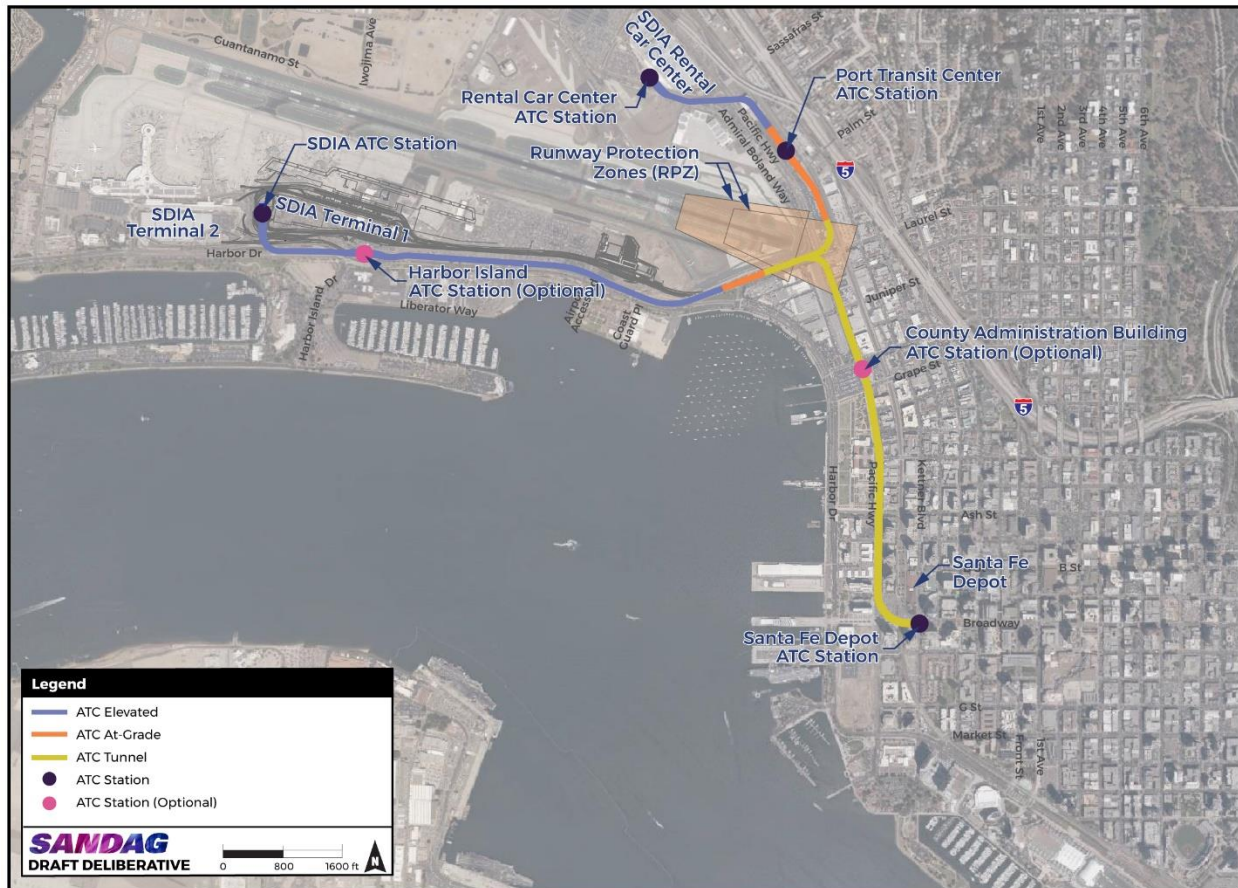
Figure 3-6. Concept 3B Bored Tunnel Airport Transit Connector from San Diego International Airport to Santa Fe Depot
