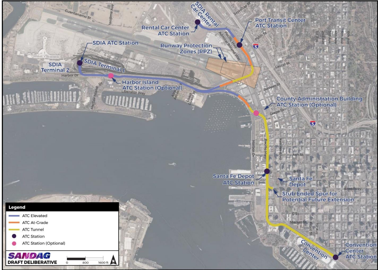
Figure 3-10. Concept 4C Hybrid Airport Transit Connector from San Diego International Airport to Santa Fe Depot Extended to Convention Center
