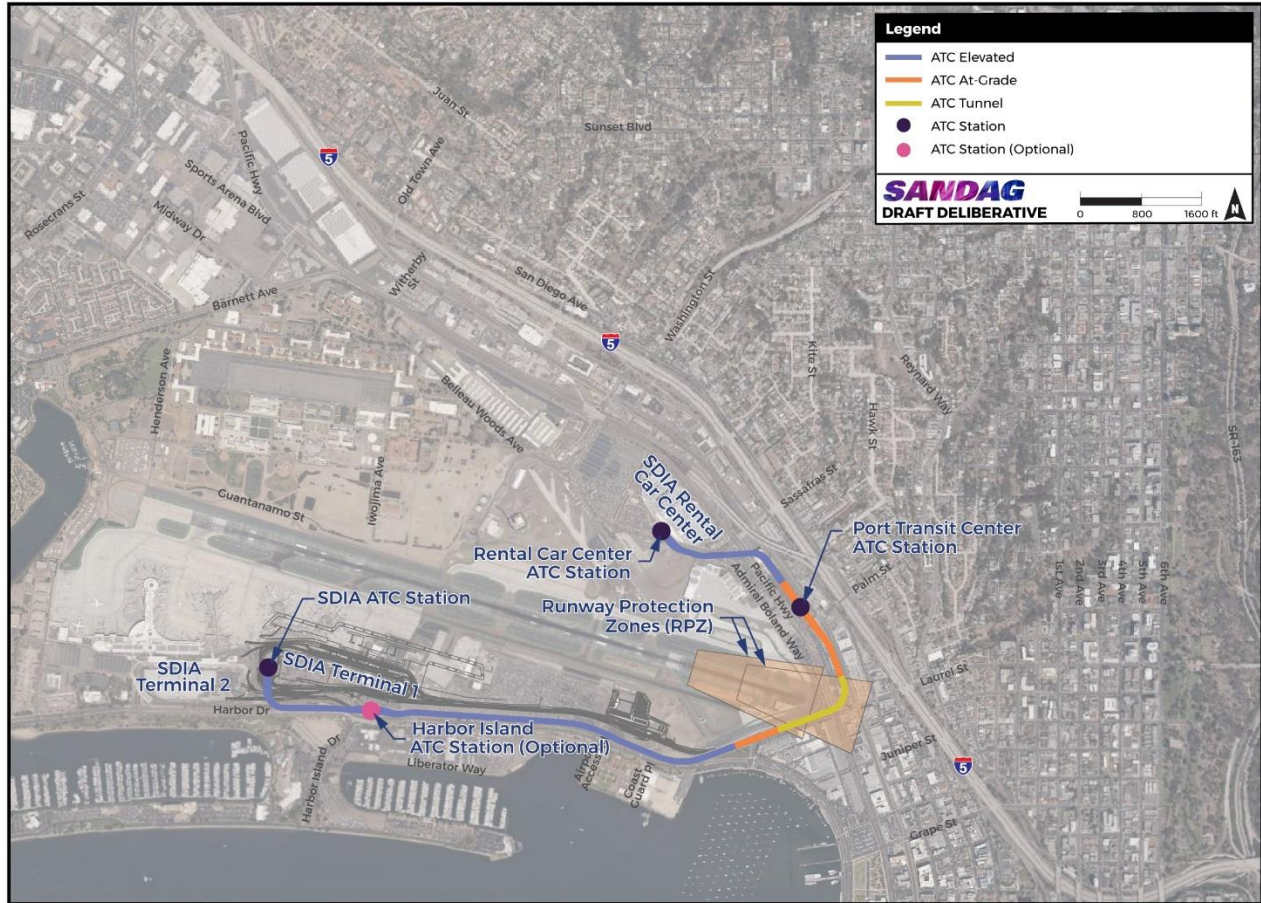
Figure 3-1. Concept 1A: Airport Transit Connector from San Diego International Airport to Port Transit Center and the Consolidated Rental Car Center
