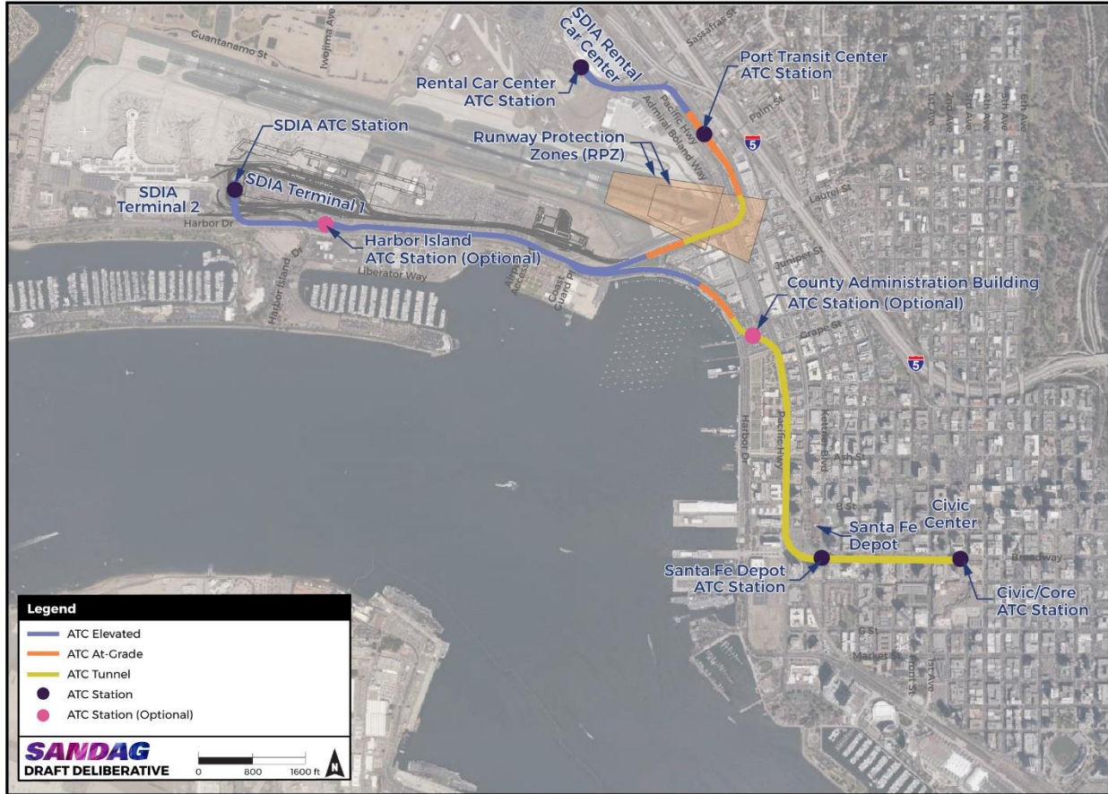
Figure 3-13. Concept 5C Hybrid Airport Transit Connector from San Diego International Airport to Santa Fe Depot Extended to Civic/Core
