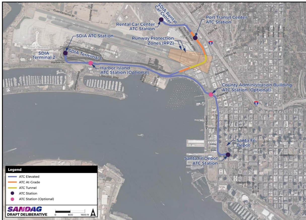
Figure 3-5. Concept 3A Aerial Airport Transit Connector from San Diego International Airport to Santa Fe Depot
