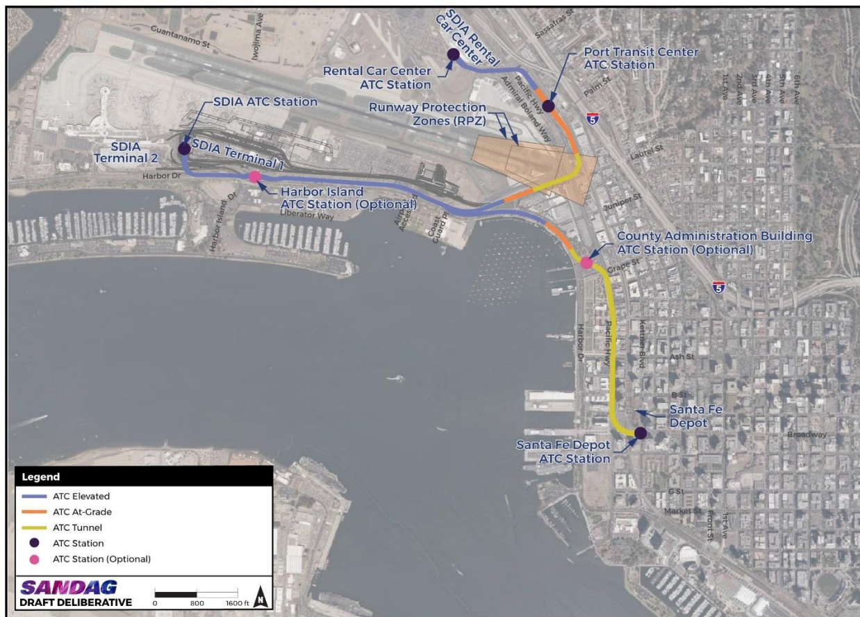
Figure 3-7. Concept 3C Hybrid Airport Transit Connector from San Diego International Airport to Santa Fe Depot
