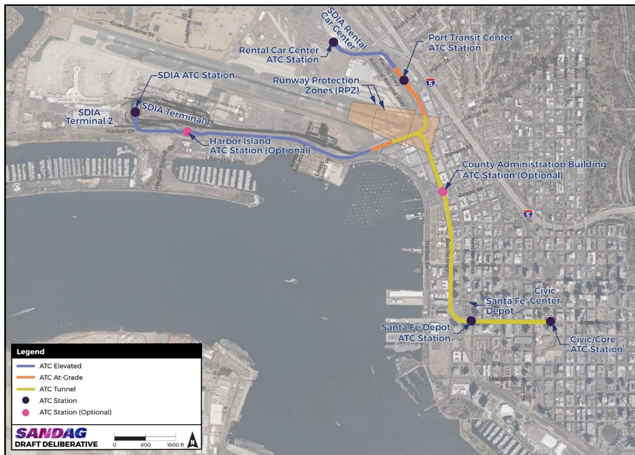
Figure 3-12. Concept 5B Bored Tunnel Airport Transit Connector from San Diego International Airport to Santa Fe Depot Extended to Civic/Core
