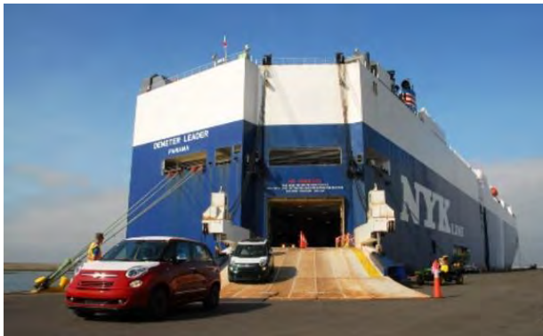
Vehicle driving of stern ramp
