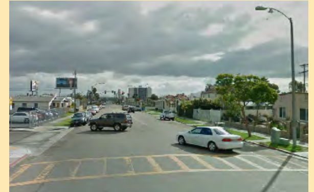
5 Uncontrolled pedestrian crossings near schools could be upgraded with more visible striping, better signage, and other pedestrian enhancements like RRFBs. Opportunity to leverage access improvements that will serve both the station and area schools.
