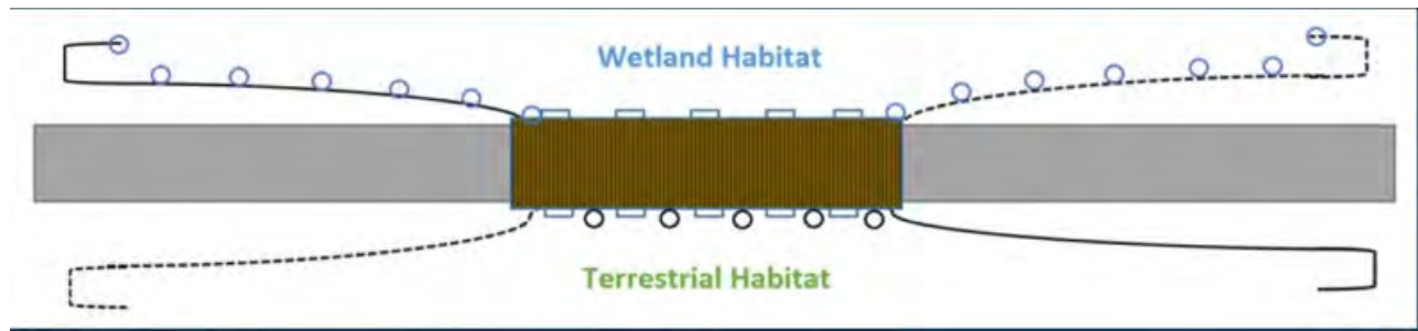
Figure 3. Schematic of Elevated Road Segment, Mesh Fencing (Dotted Lines), Solid Fencing (Lines), HALT Cameras (Circles), and Time Lapse Cameras (Black Circles); Not to Scale.
