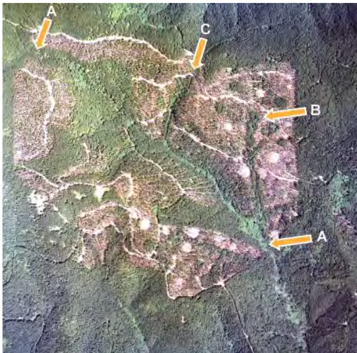
Figure 8 —Connectivity designs to aid species dispersal among ownership blocks may overlay on streamside riparian management zones. This US Bureau of Land Management study site for the Density Management and Riparian Buffer Study of western Oregon (Cissel et al. 2006) shows riparian buffers extending along the full diagonal (A) as well as laterally toward an opposing corner (B), with leave islands and dispersed tree retention aiding habitat connectivity, and to a neighboring private land block (C). “Stream-lined” connectivity (A) may aid within-watershed dispersal, but overland connectivity designs (B and C) may warrant consideration to link or “chain” habitats overland between watersheds. Photo provided by Oregon Bureau of Land Management.
