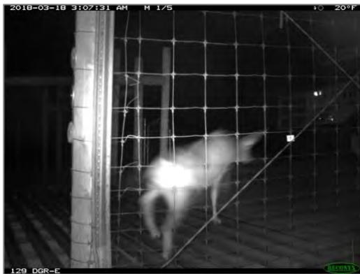
Figure 22. Mule deer breaching the Badger Road Wildlife Guard by attempting to walk on top of the round bars.
