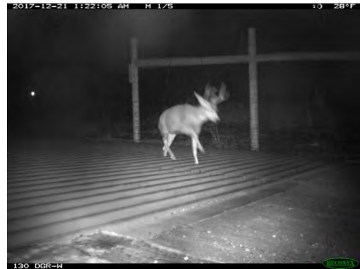
Figure 23. Mule deer breaching the County Road 1002 Wildlife Guard (round bar) by walking on the support beams.
