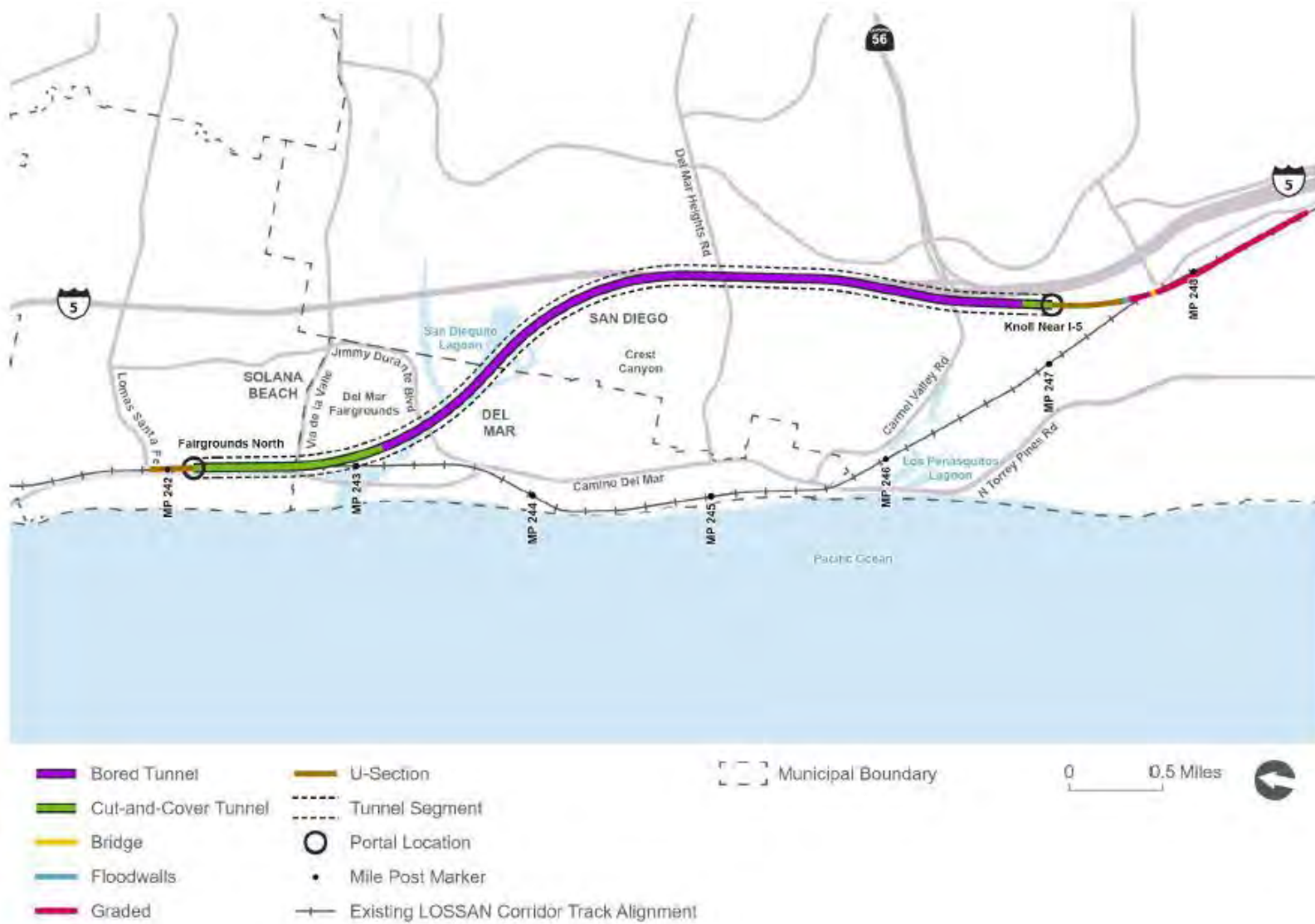
Figure 2. Alternative A alignment and design located between the Solana Beach Station and Sorrento Valley (SANDAG 2024).
