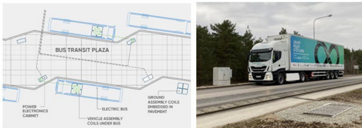
Figure 13: In-Road Inductive Charging and Static Inductive Charging (Sources: Electreon and Momentum Dynamics)
