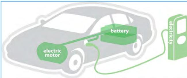
**Plug-in Hybrid Electric Vehicle (PHEV)** - Plugs into the grid and operates on electricity as well as an internal combustion engine.
