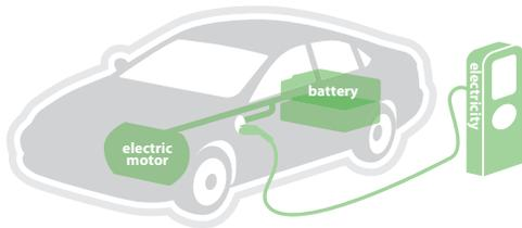
**PHEVs** are fueled by both a battery and another fuel source, usually a gasoline-powered internal combustion engine. These vehicles run on electricity from the onboard battery until the battery is exhausted and then switch to an alternate power source. PHEVs typically have a much shorter electric range than fully electric BEVs, and a standard wall outlet may be sufficient for overnight charging.
