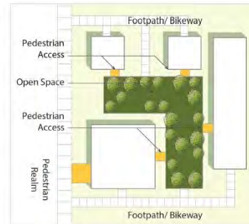
Figure 6-1 Internally accessible open space.
